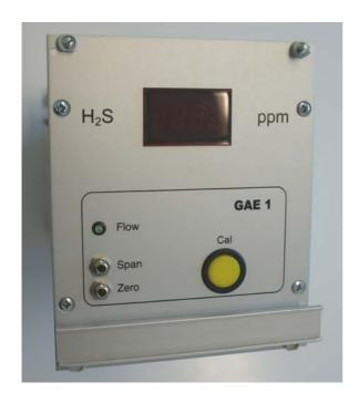
The gas analyser is provided with a chemical sensor.
